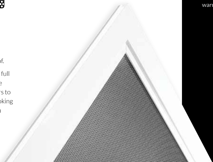
Protec's mesh is thermally treated for increased strength and performance, made from a solid 1.7mm aluminium sheet with 2.0 mm holes, providing an improved open area of 40.3% and viewing angle of 135°.
